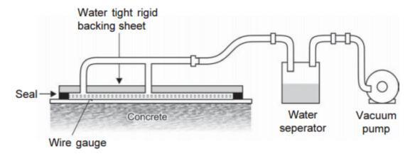
The increase in strength due to the vacuum dewatering is directly proportional to the amount of water that is removed until reaching a critical value beyond which there is no significant increase. Hence it is advised not to have prolonged dewatering expecting an increase in strength. This critical value mainly depends on the thickness of the concrete layer and the mix proportion.
