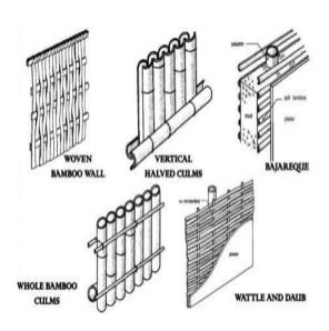
walls: Bamboo is extensively used for construction of walls and partitions. Posts and beams are the main elements normally constructed with bamboo provide a structural framework for the walls. They are positioned in a way to be able to withstand forces of nature. An infill is used between framing elements to add strength and stability to the walls.
